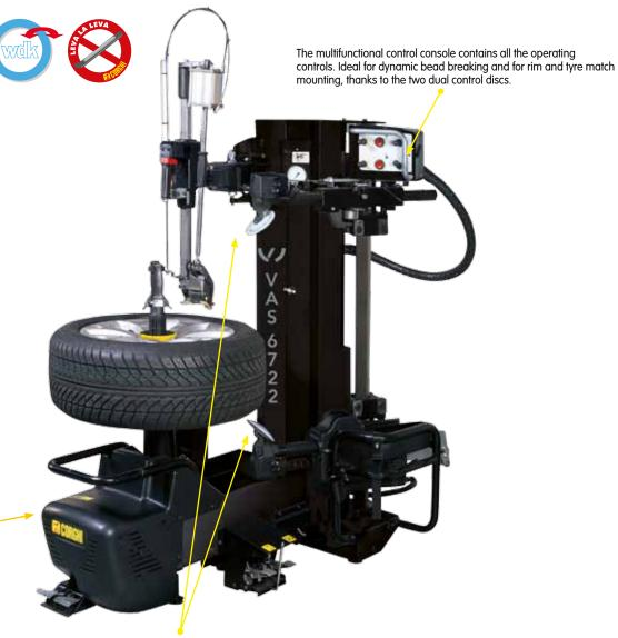
Dynamic bead breaking device with dual specular bead breaker disc. The radial positioning of the discs is made easier by automation that prevents any manual positioning errors by the operator.
